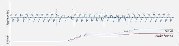
Like the proven **AutoSet** algorithm, the **Autoset Response** feature reacts to flow limitations, snore and obstructive apnoeas, but with gentler pressure increases.
